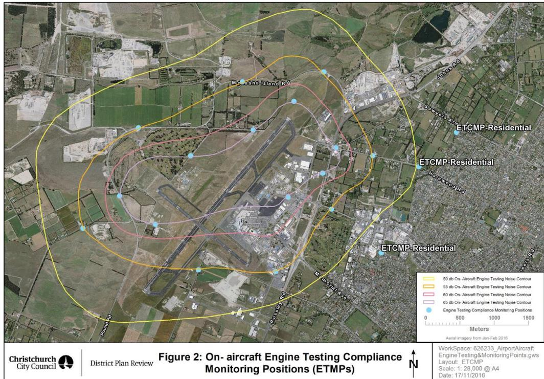
Figure 2: District Plan on-aircraft engine testing noise contours and monitoring positions
