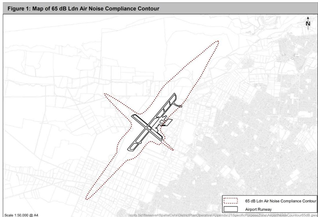
Figure 1: District Plan 65 dB  $L_{dn}$  air noise compliance contour
