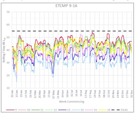
Figure 5: ETMS predicted noise levels for ETCMP 9 to 16 located on the 55 dB L<sub>dn</sub> engine testing contour
