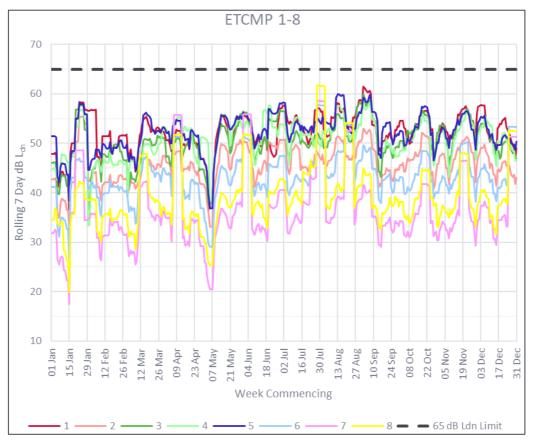
Figure 4: ETMS predicted noise levels for ETCMP 1 to 8 located on the 65 dB Ldn engine testing contour
